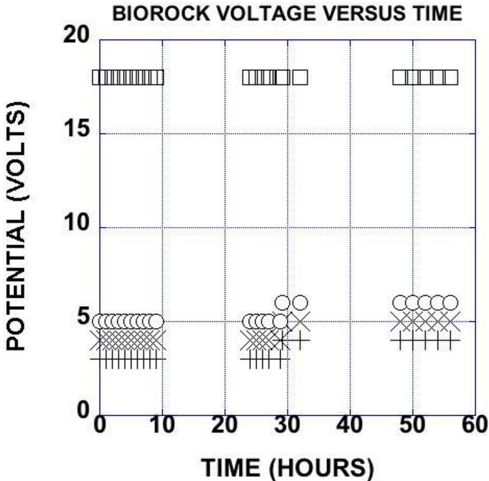
FIGURE 1. VOLTAGE OF BIOROCK PROJECTS VERSUS TIME, JANUARY 16-18, 2013. VOLTAGE WAS SET IN A CONSTANT VOLTAGE MODE, AND REMAINED STABLE. AFTER 29 HOURS THE VOLTAGES ON THE POSTS WERE INCREASED BY 1.0 VOLTS. AFTER 56 HOURS THE CHARGERS WERE CHANGED TO CONSTANT CURRENT MODE. THE + SYMBOL IS POST 1, THE X SYMBOL IS POST 2, THE O SYMBOL IS POST 3, AND THE SQUARE SYMBOL IS THE HALOPHYTE TANK.
