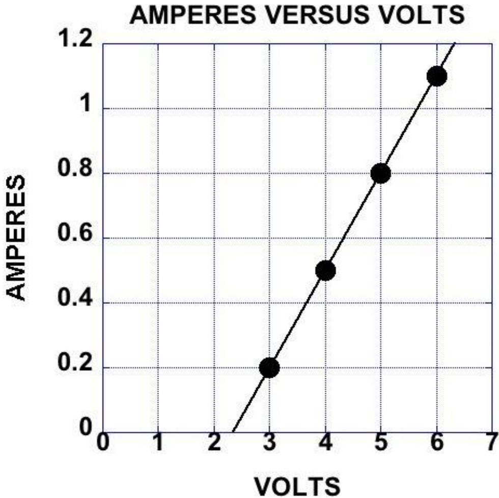
FIGURE 3. AMPERES VERSUS VOLTS FOR THE POSTS SHOWS A LINEAR RELATIONSHIP WITH A SLOPE OF 0.3 AMPERES PER VOLT, OR A RESISTIVITY OF 3.3 OHMS. THE ZERO INTERCEPT OF 2.3 VOLTS INDICATES THAT THE JUNCTION POTENTIALS PLUS VOLTAGE DROP IN THE CABLES AMOUNT TO 1 VOLT OVER THE VOLTAGE REQUIRED FOR ELECTROLYSIS OF WATER.
