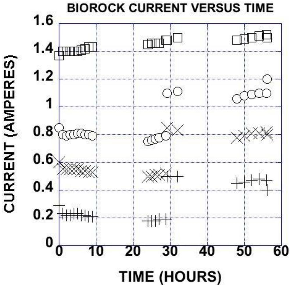
FIGURE 2. CURRENT OF BIOROCK PROJECTS AT CONSTANT VOLTAGE VERSUS TIME, JANUARY 16-18, 2013. CURRENT FLUCTUATED BY A FEW HUNDREDTHS OF AN AMPERE AS CONDUCTIVITY OF THE WATER CHANGED DURING DAILY TEMPERATURE CYCLES. AT 56 HOURS THE CURRENT WAS SET TO FIXED VALUES. SYMBOLS ARE AS IN FIGURE 1.
