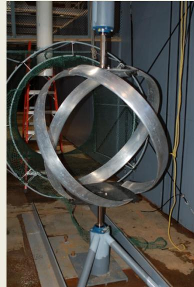
**Figure 3-** Gorlov water turbine in the Alden test flume, tapered for possible use in a pipe. Courtesy of Lucid Energy Technologies, LLP
