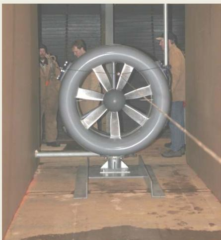
**Figure 4-** Free Flow Power turbine in the Alden test flume.
