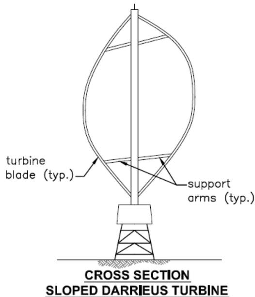
**Figure 2-** Sloped Darrieus turbine
